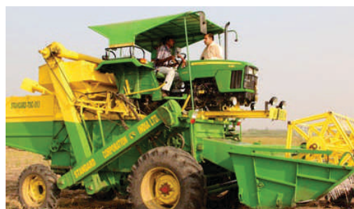
Tractor mounted combine harvester
