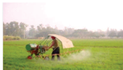
Aero blast sprayer
