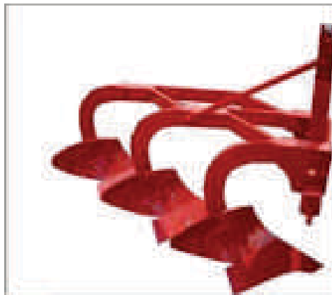
Mould-board plough
