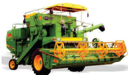
Self propelled combine harvester
